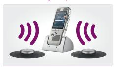
The innovative boundary layer design of the included meeting microphones uses the sound pressure of the table to provide excellent sound and recording quality with a 360 degree sound pickup radius.
